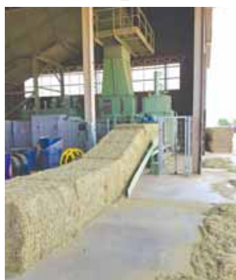
Kadant Paal balers are used for making large bales for shipment or export after hay or straw moisture has been verified.
