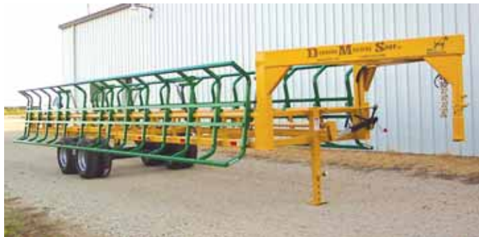
Trailers are made heavy with the cradles built from 3/16-in. metal rather than the usual 11-ga. They also bolt on for easy removal and repair, rather than being welded in place.
