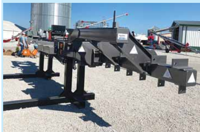
AGuru offers mounted and drawn toolbars in both 7 by 7-in. and 16 by 16-in. sizes.
