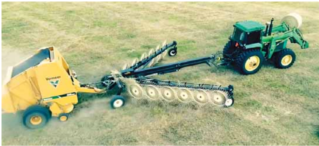
A 12-wheel Flex Rake pulling a large square or round baler can cut haying time and production costs by a third or more.
