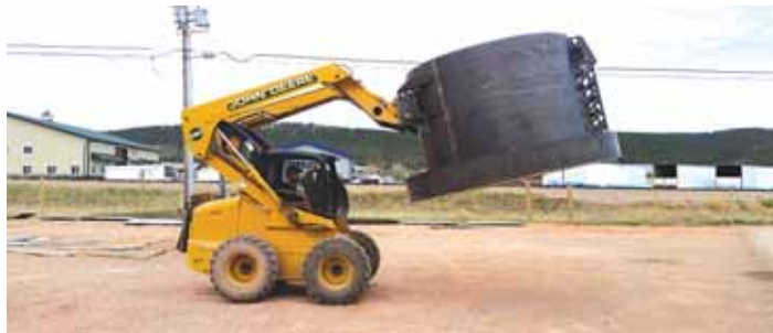
Shane Barber developed a mobile watering system made from refurbished fuel tanks that he named the Storage Drinker.
