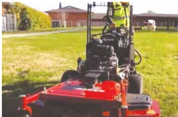
Electric Sheep Robotics makes add-on hardware that can automate a standard mower.
