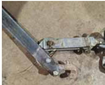
Bunniss' chain installer uses a puller and a latching device.
