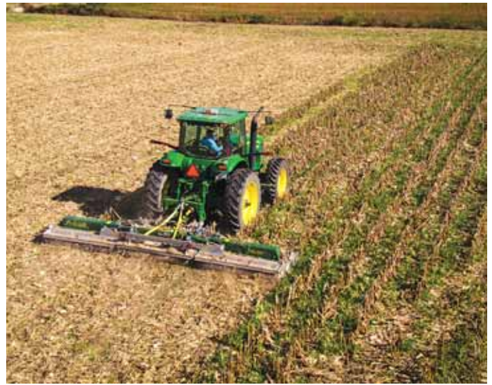
Each rotor is driven by its own gearbox without any belts or pulleys. It provides consistency of cut, even in the most challenging conditions.
