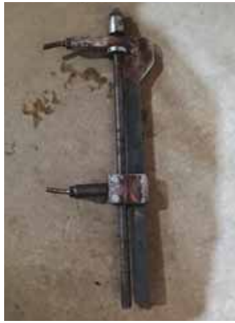
Bunniss' chain installer uses a puller and a latching device.
