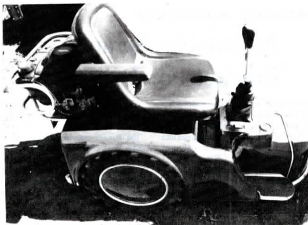
Tri-wheel chair has a hydrostatic transmission and is steered by a joystick.
