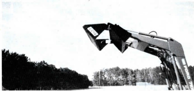
The "Hydrojaw" is a two-part loader bucket for front-end loaders.
