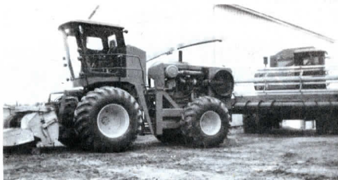
Articulated 4-WD 4-row forage harvester is powered by a Cummins 6-cylinder diesel engine and uses a high-capacity silo blower to throw silage back into a wagon.
