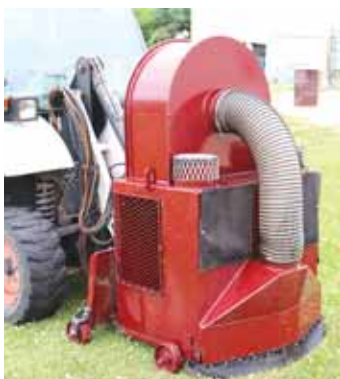
In addition to sucking up mulch, vac can be used to fill 8 or 12-in. silt socks for erosion control at the rate of 36 ft. in 50 seconds.
