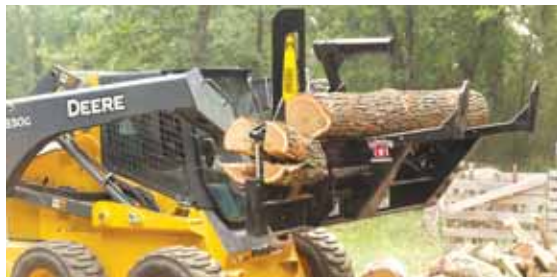
Halverson HWP-150 easily handles and cuts 22-in. logs, forcing them through either a 4 or 6-way adjustable hydraulic wedge to create perfect-sized firewood pieces.
