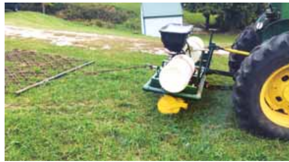
No-till grass seeder puts liquid fertilizer in the cut in the ground. "I've used it on 30 acres, and it works well. I like it because I don't have to pick it up at the end of the row," says Hodgson.
