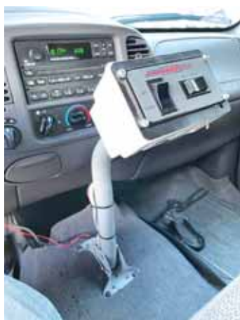
Craig Nelson raised the snowplow controls up off the floor of his pickup for easy operation.
