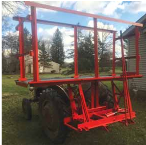
Yax modified his motorcycle lift to fit a 3-pt. hitch to make a scaffold.
