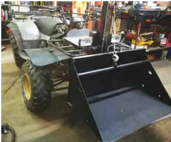
Heron's ATV modifications include a metal mower hood, plastic barrel fenders, used headlights and a winch-operated bucket.
