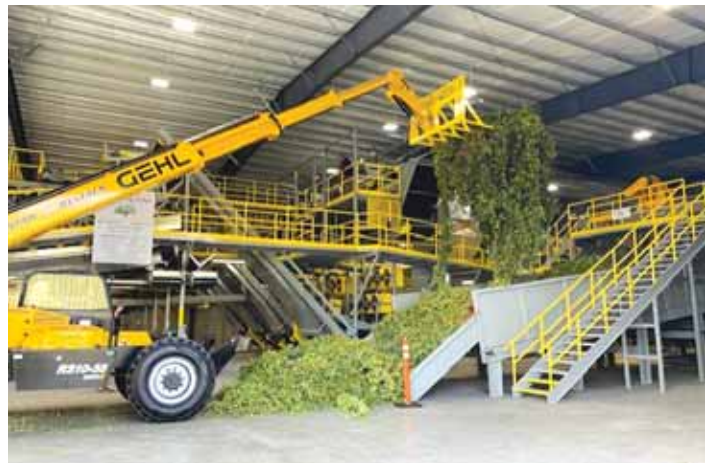
To feed hops into this equipment, telehandlers or extended fork machines are used to load and bring them by the truckload from the fields.
