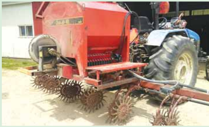
60-in. modified interseeder uses an electric seed meter and is controlled by a rheostat wired on the tractor.
