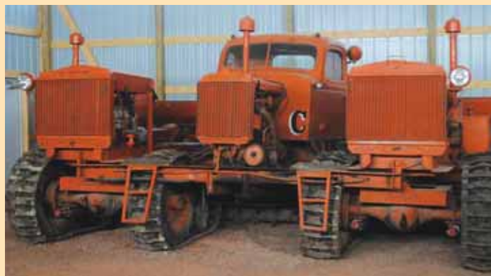
Cain built and used a self-propelled 24-ft. combination tiller/drill/packer. It was powered by three engines, including two flathead Cadillacs and an Allis-Chalmers.
