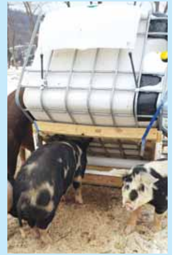
Rollers at the bottom of the tank move feed from the tote as pigs eat.
