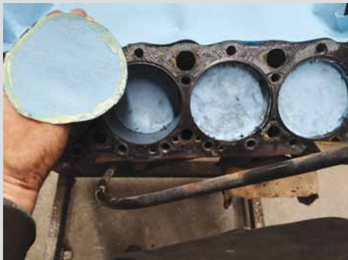
Blue shop towels with a thin layer of grease work well to keep cylinders clear of debris.
