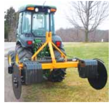
3-pt. mounted root pruner from PBW easily adapts to the orchard and its needs. The 30-in. dia., hardened, rolling disc can be set to cut up to 12-in. deep.
