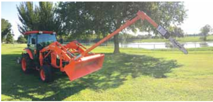
LimbSaw is equipped with a self-oiling system and a reversible motor that lets the operator back out of a pinched limb.
