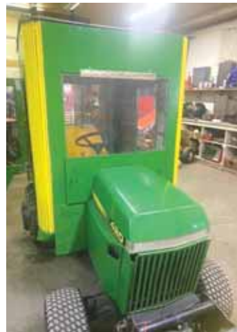
Heron built his snowblower cab from a 275-gal. tote and plywood.
