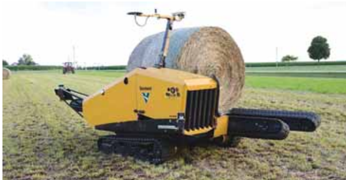
The 6,000-lb. Bale Hawk, powered by a Deutz engine, uses rubber belts to gently scoop, handle and transport three 1,400-lb. bales at a time.
