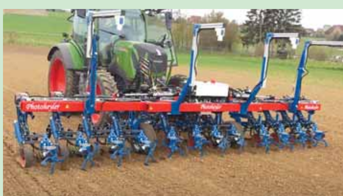
The tractor-mounted system is synchronized with the tractor wheels automatically. It detects rows and adjusts accordingly.
