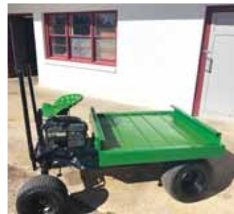
Clint Evans makes custom, motorized carts from old Murray lawn tractors.
