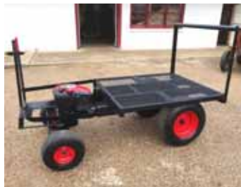
Motorized carts made from old lawn tractors with push mower engines.
