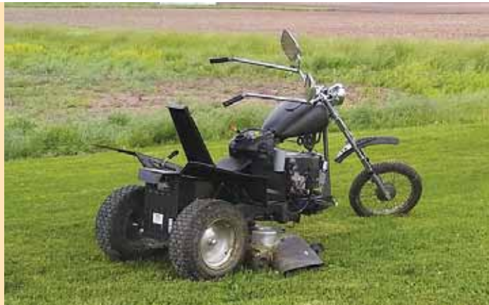
Litwiller fixed the broken axle on his riding mower and replaced it with a motorcycle front end.
