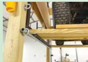
Support pipes slide through pairs of eye bolts attached to lift’s corner posts, allowing Kilby to work on mower at 2 different heights (above). Vertical angle irons fitted with small caster wheels keep mower level as it’s being raised.
