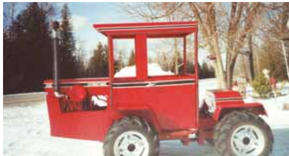
Mike Braun put two 2-WD, 125 Cub Cadets together to build this mini IH 4586 4-WD articulated tractor.
