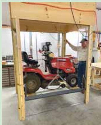
A pair of electric hoists mounted on overhead tracks are connected by cable and chains to a wooden platform that supports the mower (right). A portable workbench under the lift can be used to remove and work on the mower deck.
