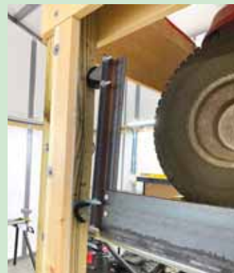
Support pipes slide through pairs of eye bolts attached to lift’s corner posts, allowing Kilby to work on mower at 2 different heights (above). Vertical angle irons fitted with small caster wheels keep mower level as it’s being raised.
