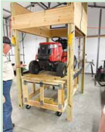
A pair of electric hoists mounted on overhead tracks are connected by cable and chains to a wooden platform that supports the mower (right). A portable workbench under the lift can be used to remove and work on the mower deck.
