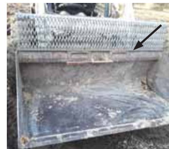
Metal grate bolted onto bucket keeps silage from spilling out. Note bolted on angle iron step.
