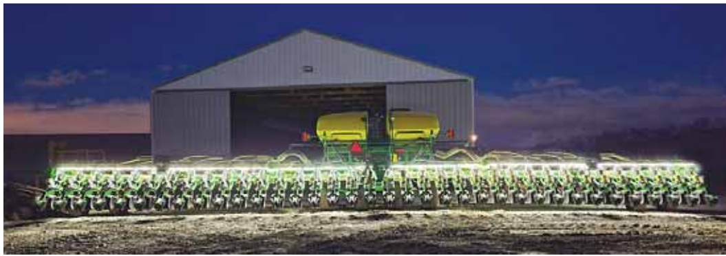
Ultra bright LED strip lights were zip tied to the vacuum tubes on this Deere 36-row soybean planter. "It's amazing how much light 900 LED's put out," says Nebraska farmer Jeremy Bacon.
