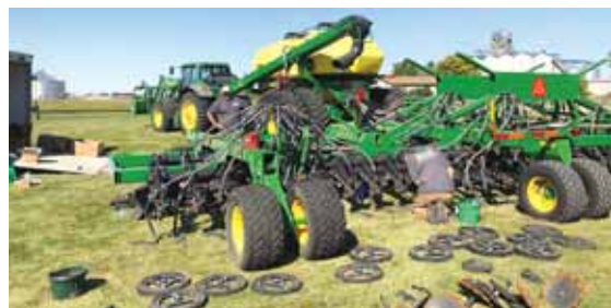
No Till Drill Services And Repair specializes in improved parts for closing wheel and press wheel pivots. Photo shows a Deere 1900 box drill rebuild.
