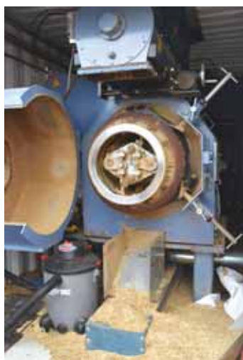
Dave Simpson uses this German-made pelletizing machine to make straw pellets for sale. Uses include everything from environmental restoration to lawn and garden mulch.
