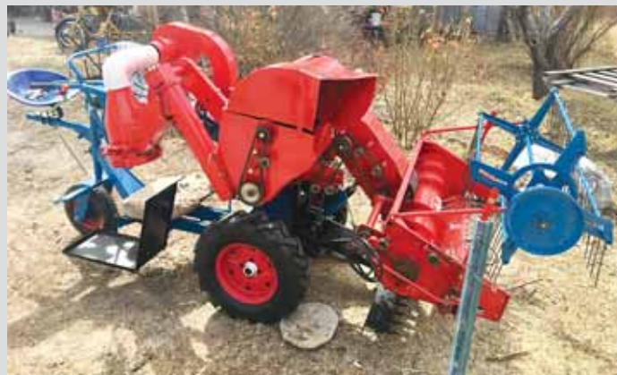
The self-propelled, mini-combine with a 3-ft. wide head and a double sicklebar can cut about an acre in 30 to 40 min. and harvest 90 to 100 lbs. of grain per hour.
