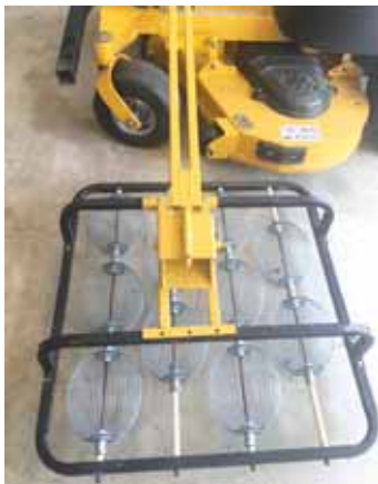
Nut Wizard mounts on side of garden tractor for use in orchards. Nuts push their way into rotating baskets.
