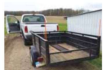
A pair of wood dowels and round magnets serve as simple trailer backup guides for Steve Faber.
