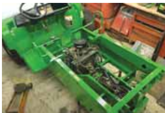
Campbell shortened the Gator frame and added a lift kit and axle extensions to match the frame to the Cub.
