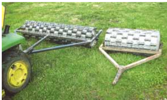
Angle iron sections welded to rollers keep them from compressing the soil.
