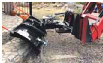
To change the angle of Chalmers' front-mounted snowplow, you just tilt the loader forward or backward.
