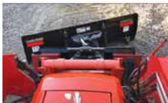
To change the angle of Chalmers' front-mounted snowplow, you just tilt the loader forward or backward.
