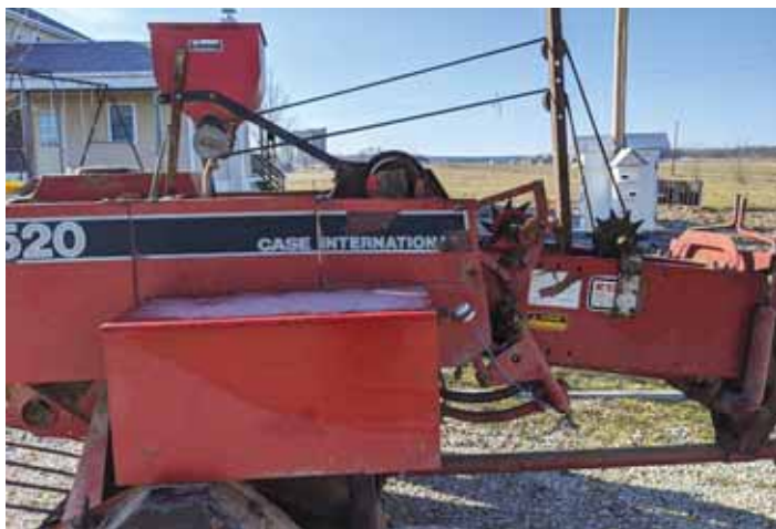
Applicator is mounted on top of baler and uses a star wheel to stop the belt and applicator when hay is not moving through baler.
