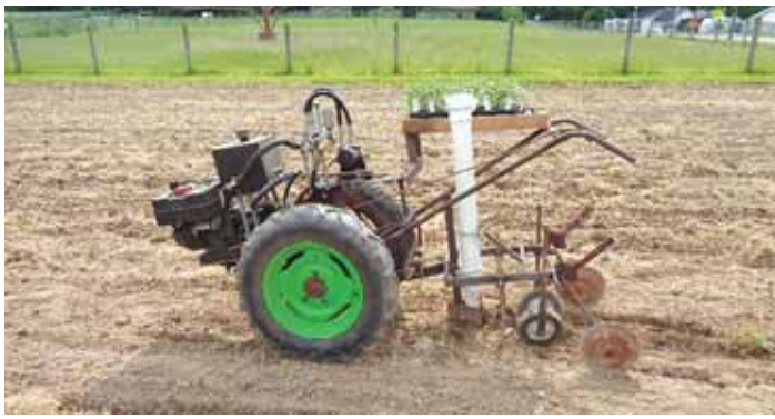
David Johnson turned an old David Brown walk-behind tractor into this one-of-a-kind tomato transplanter. "It's a lot easier than hand planting," he says.
