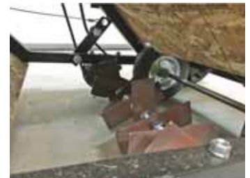
Seeder's 6-in. long blades were cut out of 2-in. wide flat bar, and are spaced 2 in. apart on a threaded rod.
