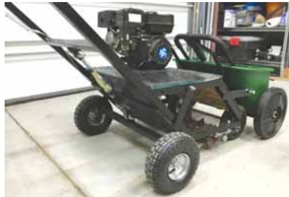
Rob Dolinski used a ground-driven drop spreader and a 5 1/2 hp. gas engine to build this belt-driven slit seeder.
