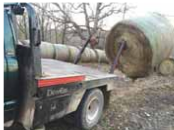
Hempel attached a 39-in. bale spear to one of the arms on truck's parallel squeeze bale bed, allowing him to stab bales placed close together in rows.
