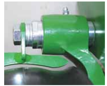
Blade mounts directly to gauge wheel arm bolt without touching tire. As planter is raised, downward tire movement dislodges any mud behind blade.
