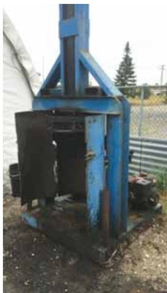
Custom-built drum crusher uses a 5-in. dia. hydraulic cylinder to flatten 55-gal. steel barrels.
