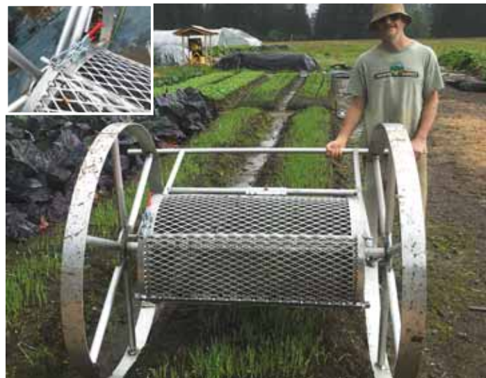
Spreader is equipped with an 18-in. dia. barrel made from expanded aluminum mesh. Inset shows toggle latches on screen's hinged loading door.
