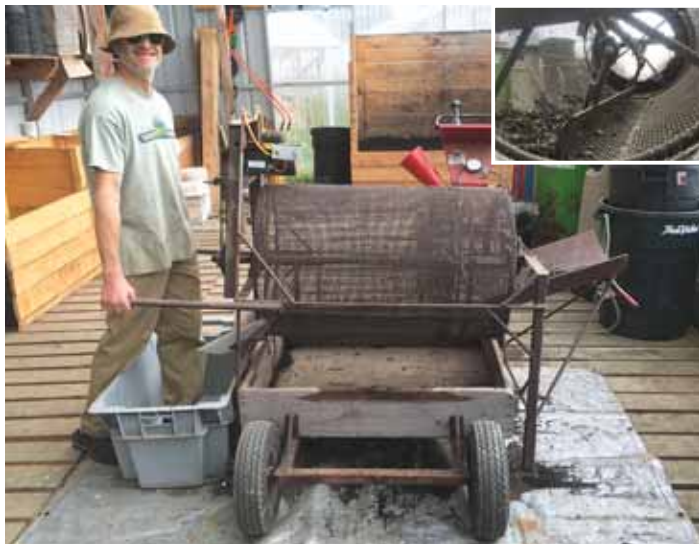
Compost sifter uses a barrel-shaped screen that rotates inside an angled framework. Sifted compost falls into a low cart. Inset shows articulated drag bar inside screen.
