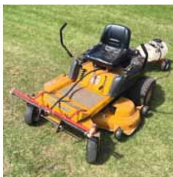
A long hose runs from trailing sprayer's tank and under mower seat up to relocated front boom.
