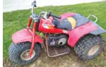
Briggs & Stratton engine chain-drives 3-wheeler's rear axle. Note homemade exhaust pipe and dummy cover on side of engine.
