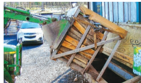
Bob Stevenson says his loader-mounted, 3-sided pallet caddies make it easy to store and move firewood.
