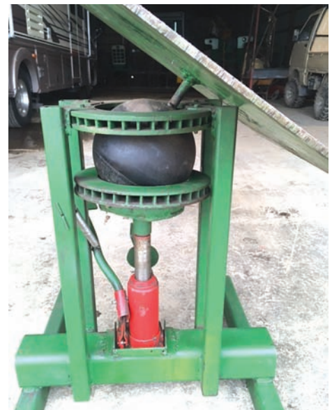
Bowling ball serves as a pivot point, allowing welding table to be easily tilted or rotated.
