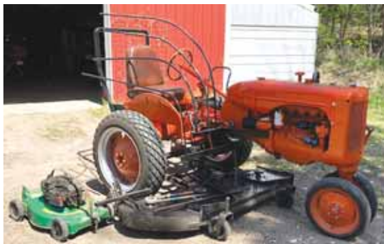
Alan "Lindy" Linda modified his Allis C for mowing around trees. He added a side mower, truck seat, custom step, and bars to move tree branches out of the way.
