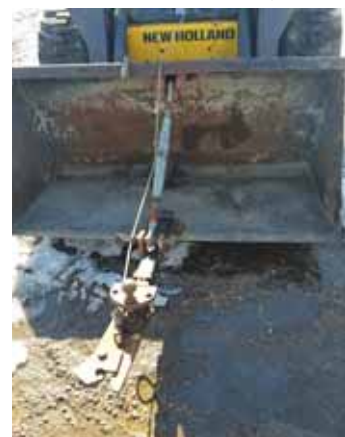
The top bracket holds a ball hitch and the bottom a spring loaded “jaw” that is operated with a rope from the cab.
