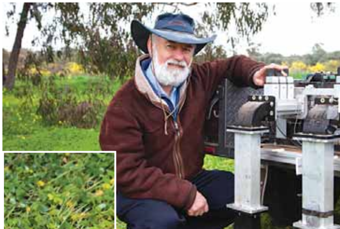
The Growave Weed Killer system uses an intense but confined microwave field to quickly heat vegetation, creating internal steam that breaks the cell walls.
