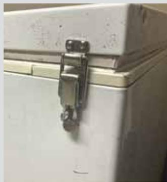
**Kylidge McNally, Bethune Saskatchewan:** “The seal was worn out on the deep freeze in our house, causing the lid not to seal properly and the inside to frost up. I put a pair of toolbox latches on the lid, one on each side, now it seals up tight.”
