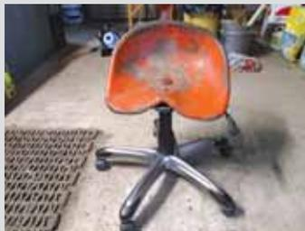
**Bern Smith, Madison, Fla.:** “I mounted an old pan-type tractor seat from an Allis WD onto the base of a discarded office chair. It rolls easily around the shop and is as comfortable as riding the Allis. It really works great.”
