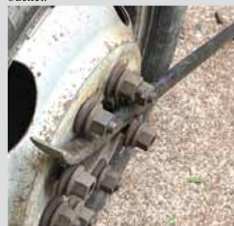
“When tightening wheel studs on truck or car tires, you can use a pry bar to hold the wheel in place. Just insert it across the wheel between the studs and rest the end on the ground.”
