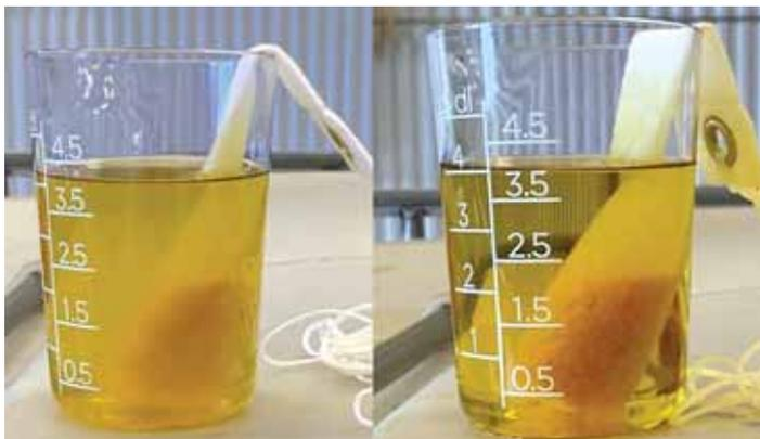
**Aquafighter® is a snake shaped pad that is inserted into a diesel fuel tank and water is trapped and removed from the fuel.**
