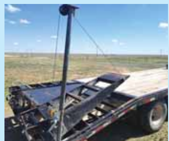
Hand crank winch makes it easy to lift ramp off trailer to ground.
