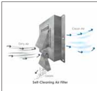
Air Cleaning Blowers work without filters. Air pressure spins particles off to the side.
