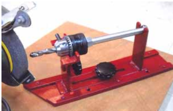
Albertson's jig lets you monitor and adjust the bit for sharpening while still in the jig, without having to remove and reposition the drill bit.
