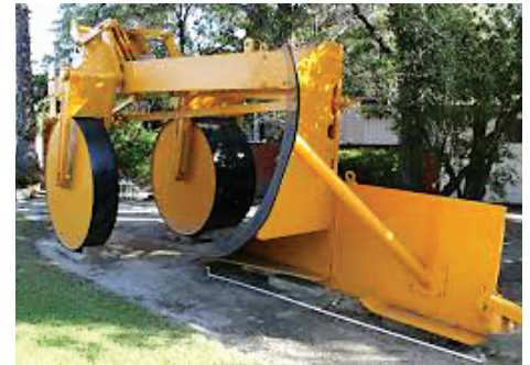
Single share, 15-ton Post moldboard plow measures 37 ft. long, 12 ft. high, and 11 ft. wide. It turned soil as deep as 7 ft.
