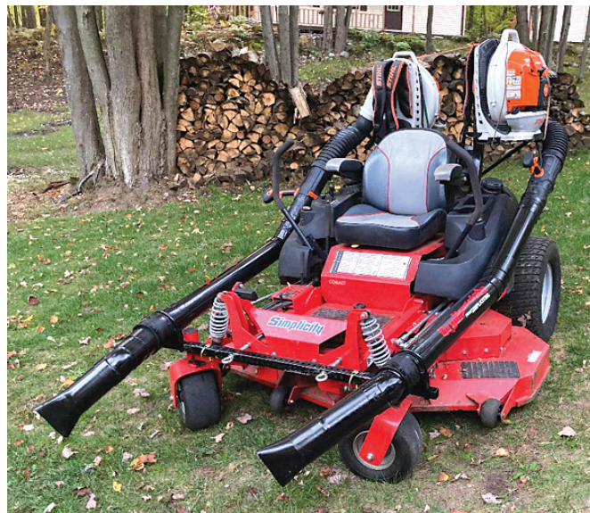
Redesigned leaf blowing system features adjustable pvc pipe mounts, rotating nozzles, and a simpler leaf blower mounting system.
