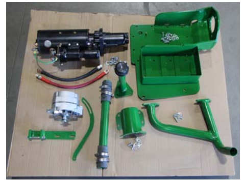
Photo shows Horning's electric start kit for Deere Model R tractors. All kits are sandblasted and painted.
