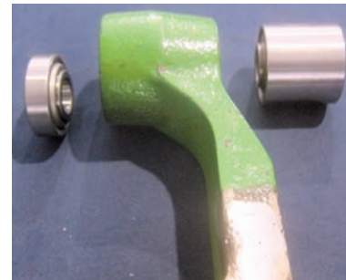
Remanufactured arms improve the performance of old and worn gauge arms by replacing the original bushings with sealed bearings.
