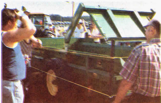
Apronless spreader features pusher blade driven by two-stage hydraulic cylinder.
