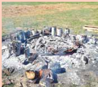
Rims were heated in a wood fire to expand enough to seal the wooden wheels when cooled.
