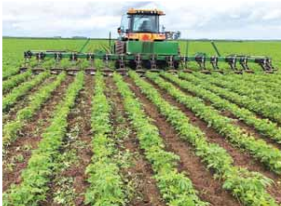
Crimping units have flexible mounts that allow for different widths by changing their angle.
