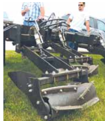
Optional blades can be bolted to the rollers for use on some crops.
