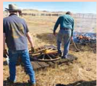
Rims were heated in a wood fire to expand enough to seal the wooden wheels when cooled.
