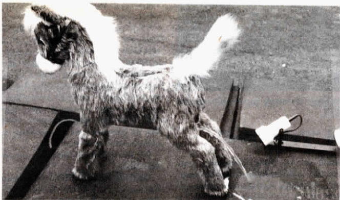
Stuffed horse demonstrates how liquid soaks right through chopped rubber flooring.
