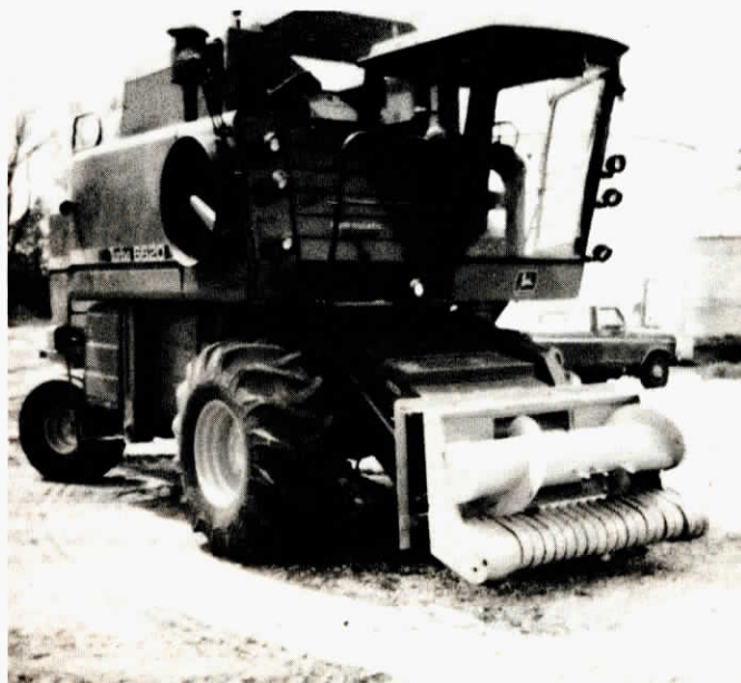
Chopper pickup is mounted directly to the combine's feederhouse. The conversion saved Hekrdle about $3,400.
