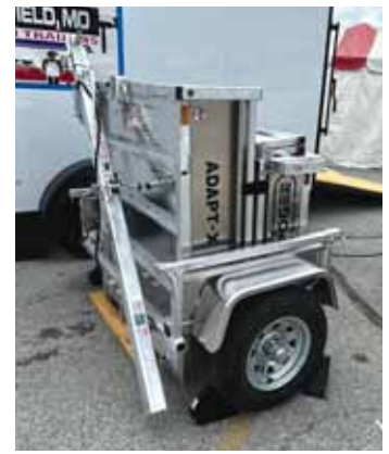
Trailer folds for easy storage and is rated for 2,990 lbs. GVWR.
