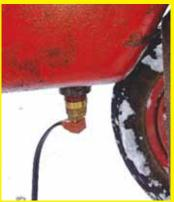
A friend gave me a Farmall with a plow to clear snow. I had an issue with water condensing in the oil every time I used it. To solve the problem, I installed a 400watt block heater on a piece of 3/4-in. pipe threaded into the drain plug hole. I plug it in for about 2 hrs. and it boils all the water out. (Rodney Corey, Johnstown, Ont.)
