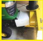
I made a shield to keep snow and ice from building up on the drive belt and pulley on my Deere 44-in. snowblower. It was made by cutting one side and the bottom out of a Rubbermaid waste basket. The flap on top of the shield is a piece of rubber inner tube that articulates when the unit is raised or lowered. The shield fits tight and doesn't need to be shield fits tight and doesn't need to be fastened to the blower to stay in place.
