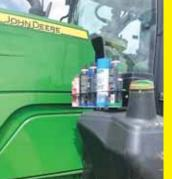
added a wire shelf to the side of my Deere tractor to hold brake cleaner, glass cleaner, WD-40, grease, and other stuff. It's attached to the toolbox and is very handy. Keeps all that stuff out of the cab (David DeLong, Wichita Falls, Texas)
