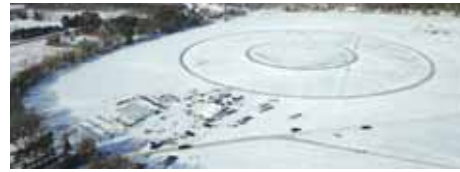
A 366-ft. dia. circle of ice spun inside a larger 820-ft. circle, both powered by small gas engines.
