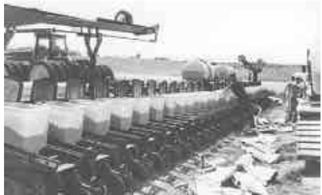
Giant planter consists of Deere vacuum planter units mounted on a Friesen toolbar. HOLDS 54 BU. SEED, 1,300 GAL. FERTILIZER
