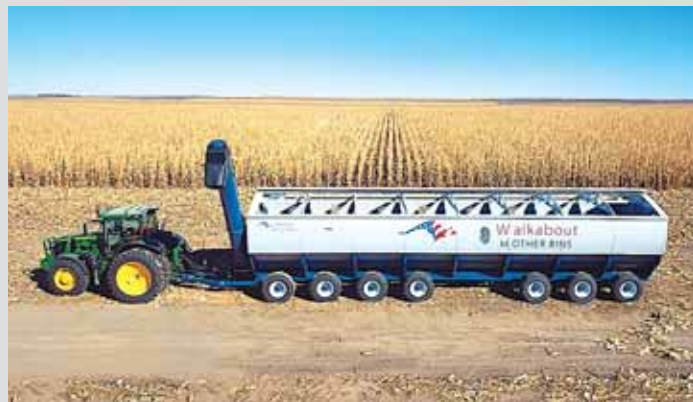
A Walkabout Mother Bin provides 4,000 bu. of portable field storage to improve harvest efficiency.
