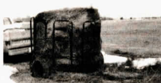
Bale is hand-winched onto the trailer bed using a rope and 4 ft. long spike.
