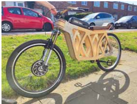
Bee designed and built an e-bike using wood and modern components.
