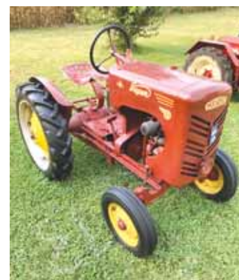
Gibson Super D with center mounted steering.
