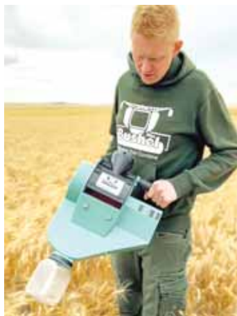
Hand-held, rechargeable device works in all grains. It contains a small thrashing drum, fan, and a choice of concaves depending on the crop being sampled.
