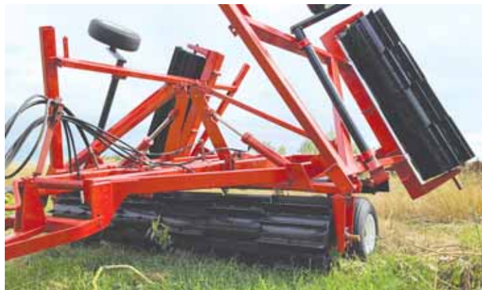
Drums were fabricated from 16-in. O.D. oil pipe found at a salvage yard. The 1/4-in. thick crimping blades extend out from the drum 4 in. Each blade was reinforced by three 3-in. by 1 1/2-in. gussets.
