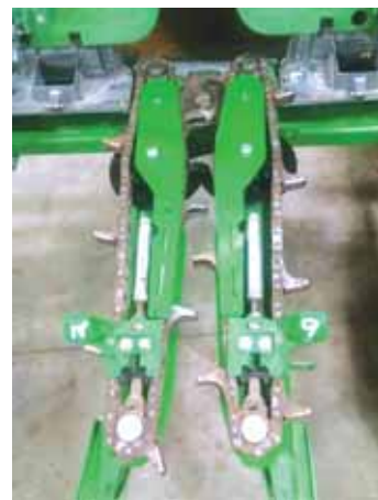
Kits contain everything required including blades, sprockets, bearings, new deck plates, chain guides, and hardware.
